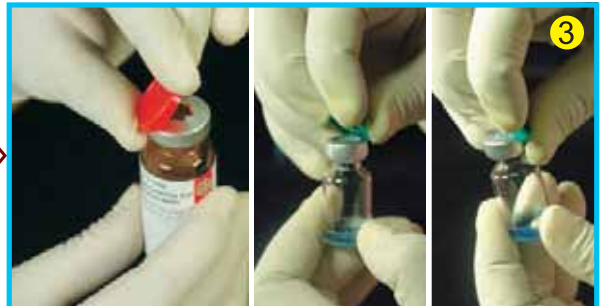
Flip off the cap of the sample vial (S-SAM), control vial (C-CTRL) and the tests (T1, T2, T3... T8).
