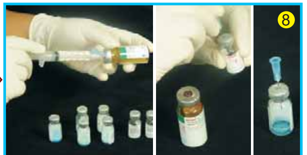
After proper mixing, draw 5 ml of test Sample from the sample vial, without any air gap in syringe (SYN-5 ml) remove the venting needle from sample vial, insert it in the slot of the control vial. and then inject 1 ml test sample in to it. Take care so that the venting needle and 18 G needle (NEE-18G) does not touch the material in the control vial.
