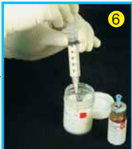
Collect 5 ml of milk sample from the milk container with the help of 5ml syringe (SYN-5ml).
