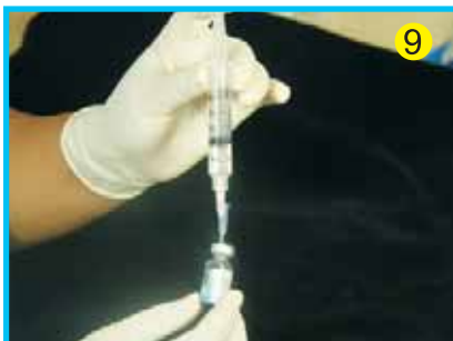
Like wise transfer 1 ml of test sample into test vials T1, T2, T3, T4 taking care to insert the venting needle in each of test vial prior to injection of the test sample.
