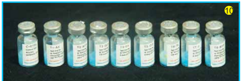
Now again draw 4 ml of the test sample from the sample vial using the same syringe and inject 1 ml each into the test vials T5, T6, T7 and T8. Once all the test vials and control vials are injected with the test sample shake the vials to mix the contents and incubate at room temperature (25-30°C) or in an incubator (35-37°C, if available) for 16-24 hours.
